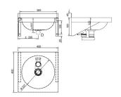
G 1/2" 1 - 10 Bar (12 V version), 2 - 8 Bar (6 V version) 12 V, 50 Hz (AUM 023.1, 023.2, 023.TV) ZAC 1/50 - max. 8× AUM 023.1, 023.TV, max. 5x AUM 023.2 6 VA, (10 VA by AUM 023.2) ZAC 1/20 - max. 3× AUM 023.1, 023.TV, max. 2x AUM 023.2
